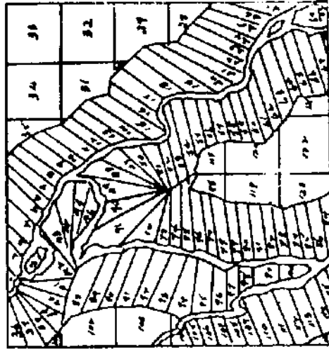
DIAGRAM OF A TOWNSHIP PLAT 6 MILES SQUARE CONTAINING 125 SECTIONS SHOWING RADIATING LOTS OR SECTIONS —BORDERING NAVIGABLE WATERS
